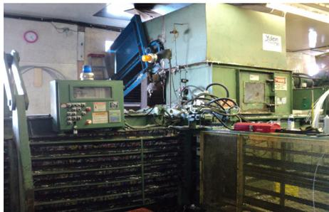
That piece of ironmongery in the picture is our baler. The baler uses the same technique as squashing a can by stepping on it, just on a larger scale. The machine squashes multiple cans (or other products)
